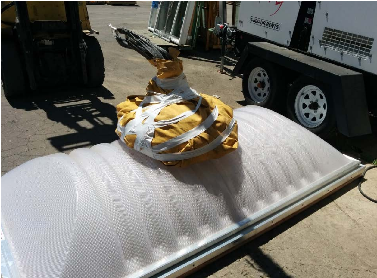
Photo No. 2 Skylight after Drop Test
